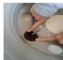
EXAMPLE OF VALVE STEMS INSTALLED OPPOSITE OF EACH OTHER IN A SPRINTER STEEL WHEEL. DUALYVALVE KIT PN#DL1SP13
