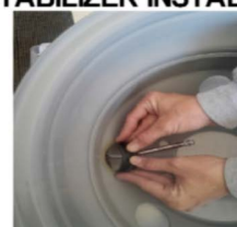
EXAMPLE OF VALVE STEMS INSTALLED OPPOSITE OF EACH OTHER IN A SPRINTER STEEL WHEEL. DUALYVALVE KIT PN#DL1SP13
