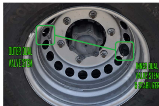
EXAMPLE OF VALVE STEMS INSTALLED OPPOSITE OF EACH OTHER IN A SPRINTER STEEL WHEEL. DUALYVALVE KIT PN#DL1SP13
